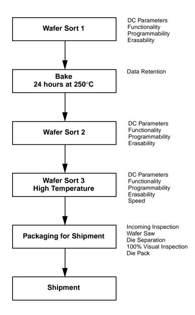
Figure 1. AMD KGD Product Test Flow
